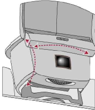
2. Focus the camera by turning the focus wheel:
